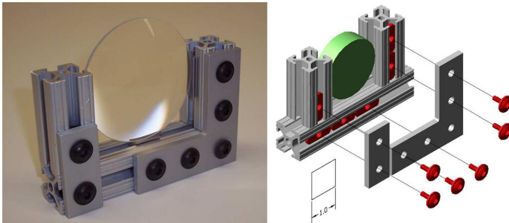
**Figure 2.** Mount for 3 inch diameter achromatic condenser lens.
