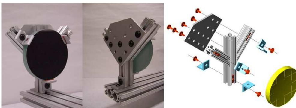
**Figure 4.** Front and back views of mount for 4.5 inch diameter mirror. Small pieces of soft rubber are used to cushion the mirror at the three points where it is held by the mount.
