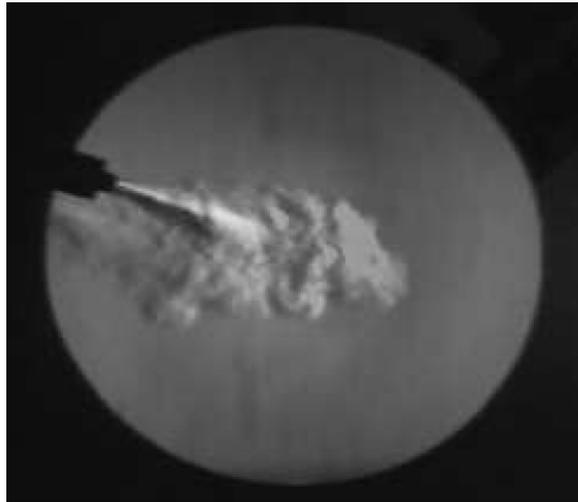
**Figure 9.** Schlieren image of a jet of helium gas taken with the prototype single-mirror system (figures 6(c) and 7). The large dynamic range of the image and the low bit-depth of the camera (8 bits) causes many parts of the image to be saturated.
