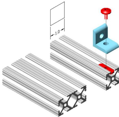
**Figure 1.** 80/20 assembly. Figure demonstrates how 10 series T slotted rods are connected to a 'joining plate'. Rods are classified according to their cross-sectional area. A 1010 ( $1 \times 1 \text{ inch}^2$ ) and 1020 ( $1 \times 2 \text{ inch}^2$ ) rod are shown.
