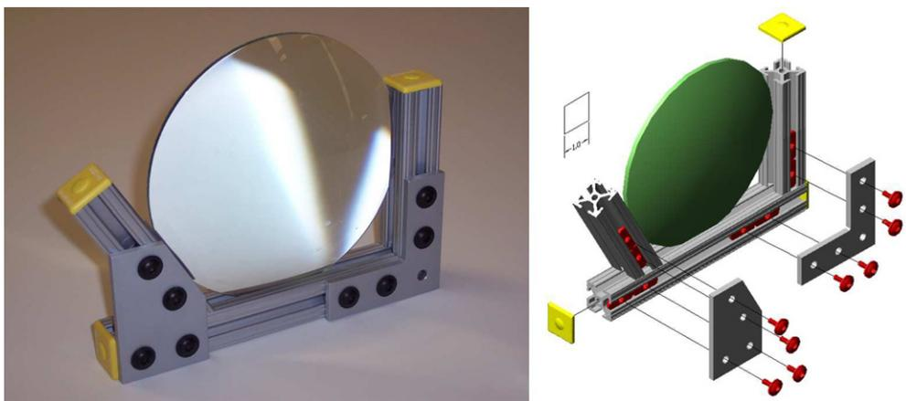
**Figure 3.** Mount for 6 inch diameter schlieren field lens (see figure 6(a)).
