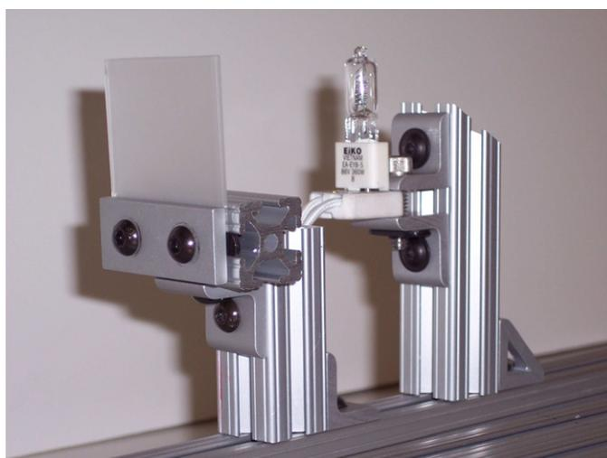
**Figure 5.** A simple mount for a lamp and a filter holder. The filter is a square, 2 inches on a side.
