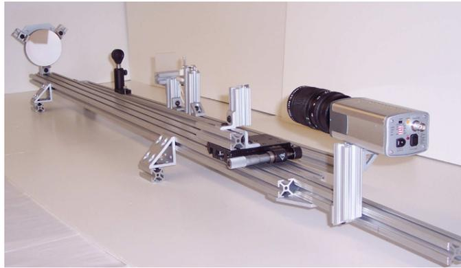
**Figure 7.** The final single mirror schlieren setup (figure 6(c)). The knife edge is seen mounted on a translation stage. The pinhole has been moved further away from the diffuser for clarity. During operation, the diffuser is placed as close to the pinhole as possible.
