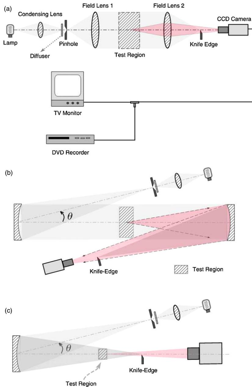
**Figure 6.** Schlieren imaging configurations: (a) a two-lens, in-line system, (b) a two-mirror, Z-type system and (c) a single mirror system. The test region is shown hatched in all figures. Typical ray paths imaged by the camera are shown in red.
