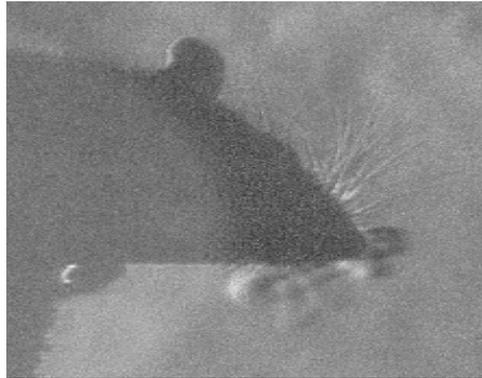
**Figure 8.** Schlieren image of air exhaled from a deeply anesthetized rat. The image was taken with a single mirror schlieren system that used a 12 inch diameter mirror and a high speed camera (Photron Fastcam-1024PCI, 1 KHz frame rate). The slightly brighter semi-circular region in the image is light reflected from a beam-splitter.
